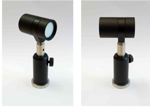
Fig. 4: Mounting option: FTL-f32.5mm and CTL-D25mm mounted with SMR1
