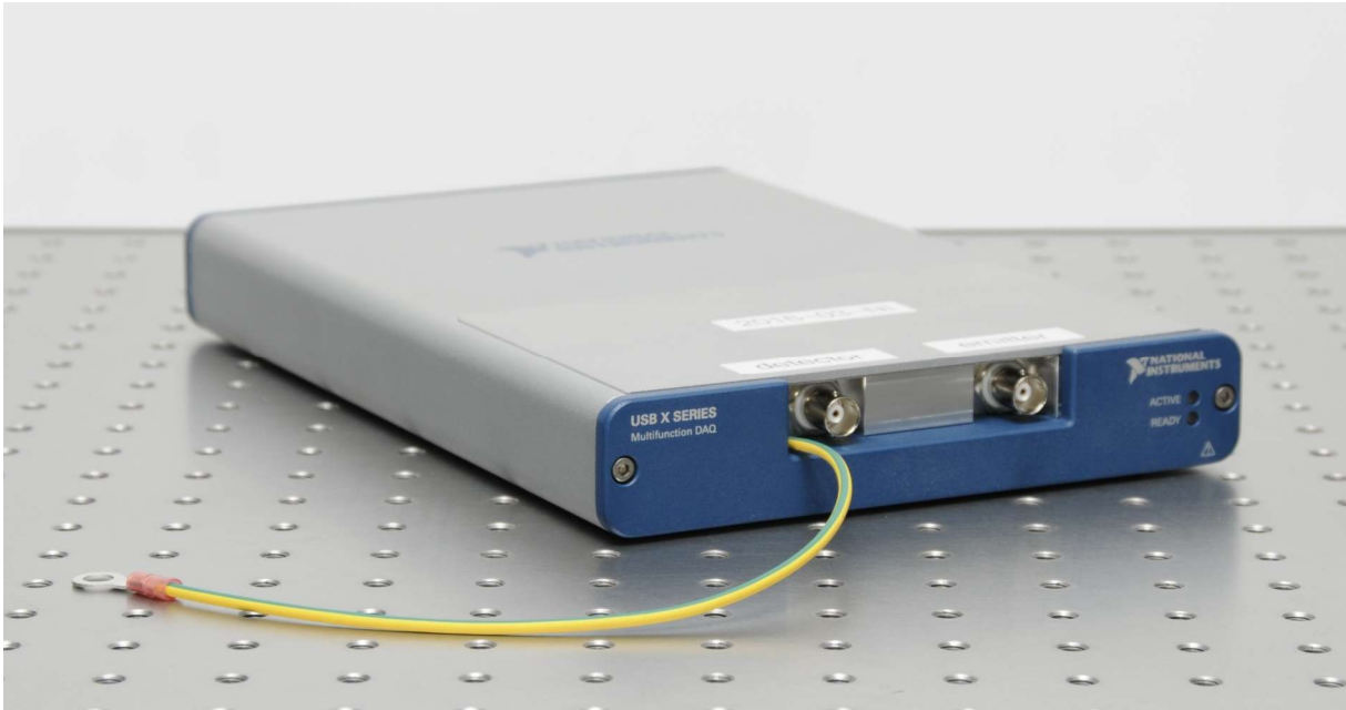
Figure 2: Data acquisition systems with BNC ports for emitter and detector antenna.
