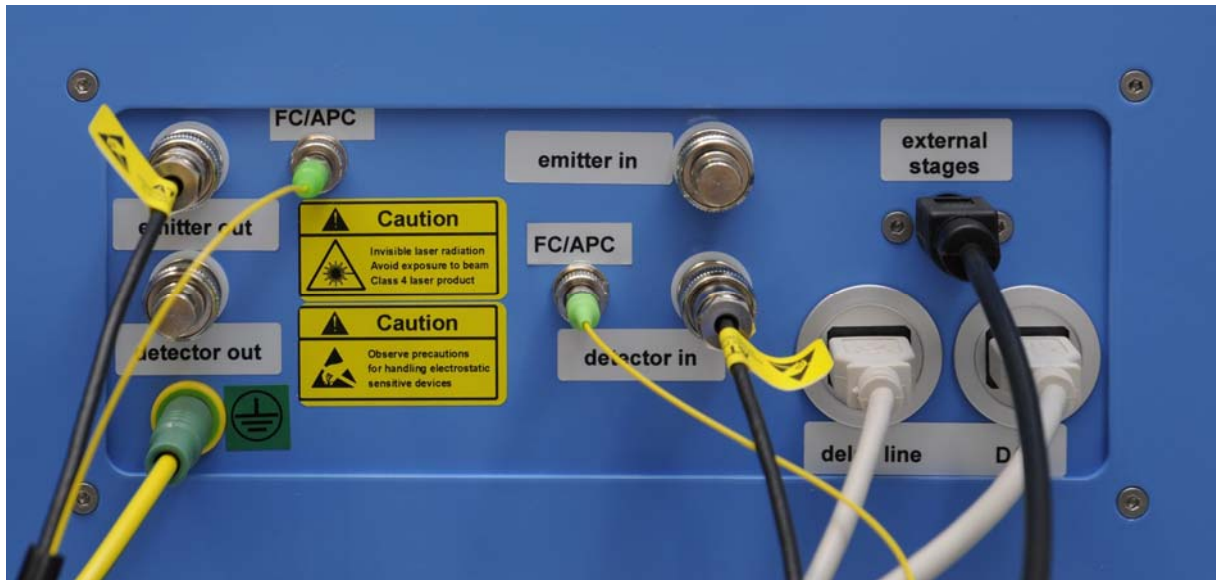
Figure 12: Panel on the right hand side of a TDS system with ports for electrical and optical connection of THz antennas, external stages (imaging unit or angular scanning unit), the delay line and the data acquisition system (DAQ). The panel shown is configured for the use of the external fiber-coupled antennas.
